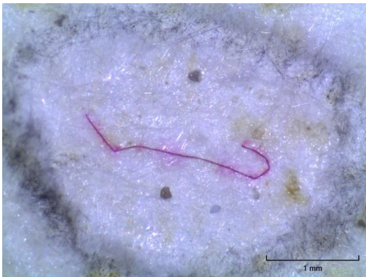
Figure 19. Example of cellophane/rayon fibre with colour seeming to be leaching of after KOH-treatment.
